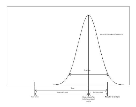
The validation and quality control tools are used to evaluate the systematic errors and the random errors, and to monitor their changes over time.
