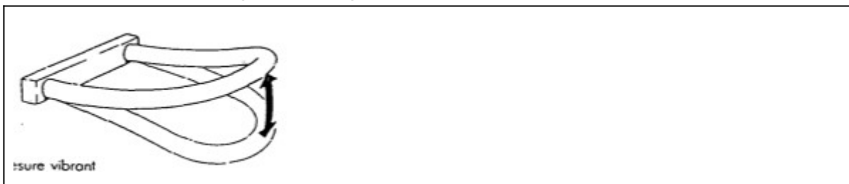
Figure 1: Vibrating measuring tube
