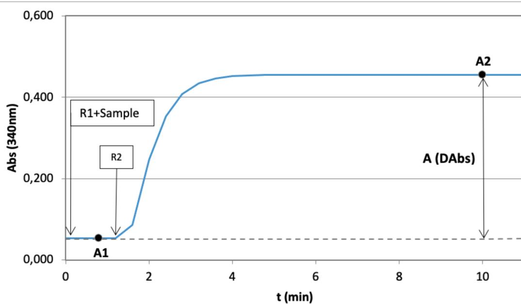
Figure 1: Example of reaction kinetics
