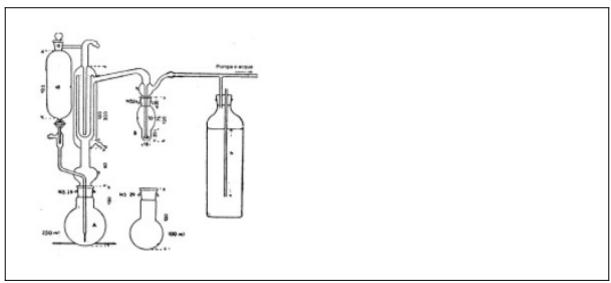
The gas feed tube to the bubbler B ends in a small sphere of 1 cm diameter with 20 0.2-mm diameter holes around its largest horizontal circumference. Alternatively, this tube may end in a frit glass plate which produces a large number of very small bubbles and thus ensures good contact between the liquid and gaseous phases.
