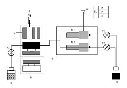
A: differential amplifier; B: buffer solution; C: mixing chamber; D: indicator;  $EL_1$  and  $EL_2$  capillary electrodes; EL: electronics; G: ground; K: keyboard; M: magnetic stirrer; P: printer;  $P_1$  to  $P_3$ : peristaltic pumps; S: injection syringe for the sample and enzyme; W: waste.
