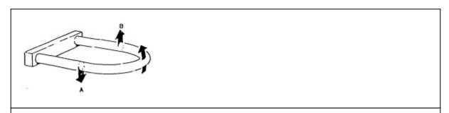
Figure 2: Reactive forces exerted by the fluid
