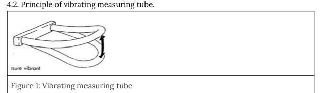
Electronic densimeters operate according to the vibrating measuring tube principle (fig. 1): the fluid is introduced into a U-shaped tube and subjected to electromagnetic excitation (fig. 2 and fig. 3).
