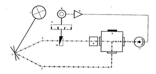
A light source (1) powered by the electricity network projects a beam of light onto an oscillating mirror (2) which alternately reflects a measuring beam (3) and a comparison beam (4) at a rate of approximately 600 times per second.
