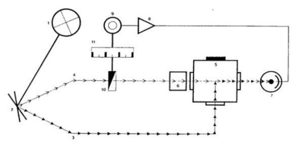
A light source (1), powered by the mains, sends a beam of light onto the oscillating mirror (2) which reflects alternatively a measuring beam (3) and a comparison beam (4) about 600 times per second.
