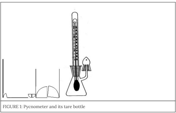
This pycnometer includes a side tube of 25 mm in length and an inside diameter of at most 1 mm, terminated by a ground-glass conical joint. This side tube may be capped by a 'reservoir stopper' composed of a ground-glass conical tube, terminated by a tapered joint. This stopper serves as an expansion chamber.
