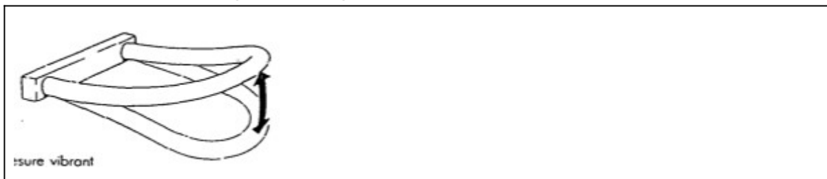
Figure 1: Vibrating measuring tube
